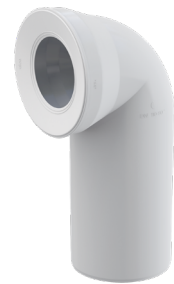
A90-90A Connector for floor-standing WC, 90° elbow, DN 110, length 230 mm, PP, white
