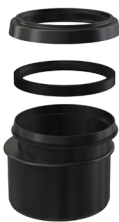
M907 Waste reducer for wall-hung WC, eccentric 7 mm, DN 90 x DN 110, length 98 mm, PE, black
