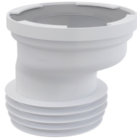
A991-20 Connector for floor-standing WC, eccentric 20 mm, 110 mm, length 125 mm, PP, white
