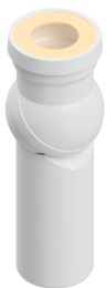
A90-90R Connector for floor-standing WC, adjustable elbow 0–90°, DN 110, length 275 mm, PP, white
