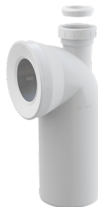
A90-90P40/50A Connector for floor-standing WC, 90° elbow with DN 40/50 inlet, DN 110, length 230 mm, PP, white
