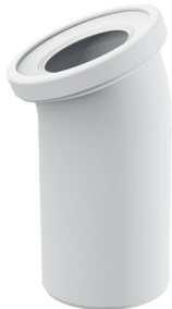
A90-22 Connector for floor-standing WC, elbow 22°, DN 110, length 165 mm, PP, white
