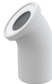
A90-45 Connector for floor-standing WC, 45° elbow, DN 110, length 90 mm, PP, white
