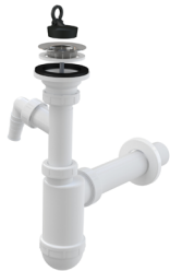
A41P Washbasin trap DN 40 with Ø 17–23 mm connector and stainless steel grid Ø 62 mm, rubber plug
