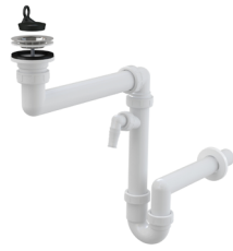
A870P-DN40 Sink waste and trap DN 40 space-saving with \varnothing 17–23 mm connector and stainless steel grid \varnothing 70 mm, rubber plug
