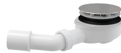
A491CR Shower waste and trap, reduced height, waste outlet 90 mm, DN 50, plastic, chrome-polished
