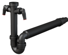
A84-DN50/40-ECO Tubular sink waste and trap DN 50/40 with two Ø 17-23 mm connectors, G 6/4" union nut and flexible hose
