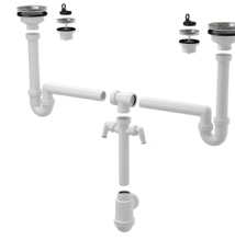
A8000 Double-sink waste and trap DN 40/50 universal, with two \varnothing 17–23 mm connectors, stainless steel grids \varnothing 70 mm and \varnothing 115 mm, rubber plug
