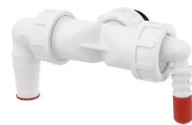
P156Z-G1 Double connector G 1" \times \varnothing 8–23 mm for connecting washing machine and dryer to trap, with non-return valves
