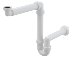
A434 Washbasin trap DN 40 space-saving with G 5/4" union nut
