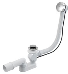
A55K Bath pop-up waste and trap, length 57 cm, metal, chrome-polished
