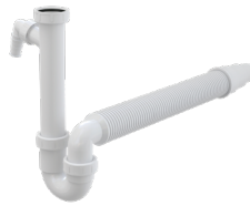
A83-DN50/40 Tubular sink waste and trap DN 50/40 with \varnothing 17–23 mm connector, G 3/4" union nut and flexible hose
